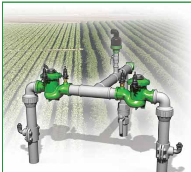
[1] BERMAD Model IR-972-M0-2W-KVZ limits over-demand, controls laterals and distribution line fill-up while reducing pressure, and measures flow.
