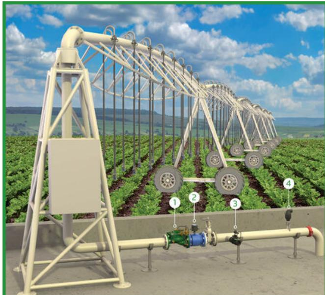
[1] BERMAD Model IR-420-55-3W-RX opens in response to electric signal, and establishes reduced pressure zone protecting laterals and distribution line.
