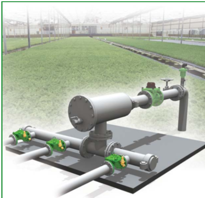
[1] BERMAD Model IR-420-54-R opens upon pressure rise command, establishing reduced pressure zones.
