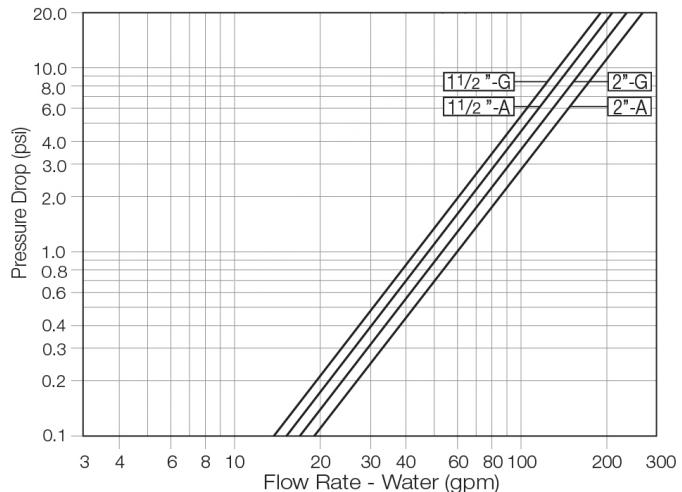
2-Way circuit "Added Head Loss" (for "V" below 6.5 f/s): 4.5 psi
