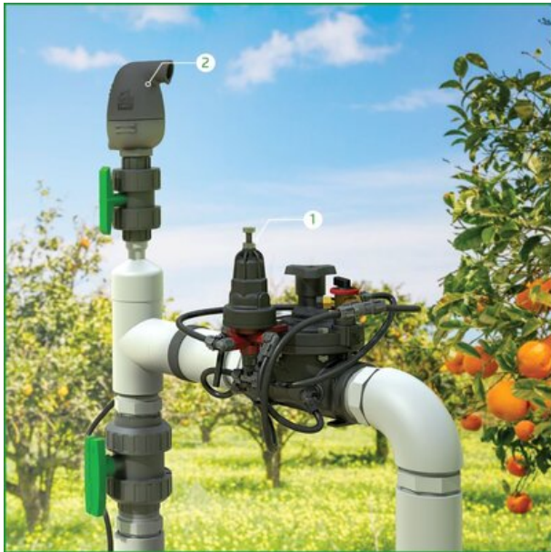
[1] BERMAD Model IR-220-50-3W-XZ Opens upon pressure drop, and establishes reduced pressure zone protecting laterals and distribution line.
