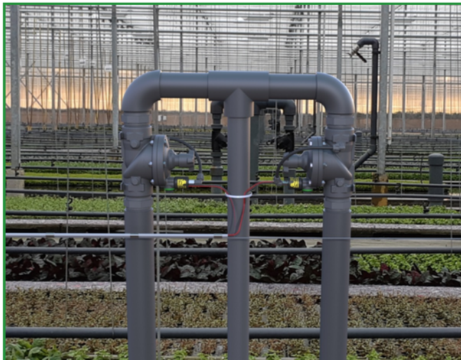
[1] The BERMAD Model IR-21T-N6-2W-M opens and closes drip-tight in response to an electric signal, which causes the solenoid to open or close the valve's internal hydraulic loop.
