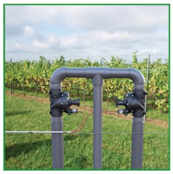
The BERMAD Model IR-21T opens and closes drip-tight in response to an electric signal, which causes the solenoid to open or close the valve's internal hydraulic loop.
