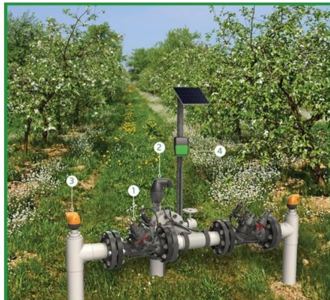
[1] BERMAD Model IR-120-55-3W-X opens in response to electric signal, and establishes reduced pressure zone protecting laterals and distribution line.
