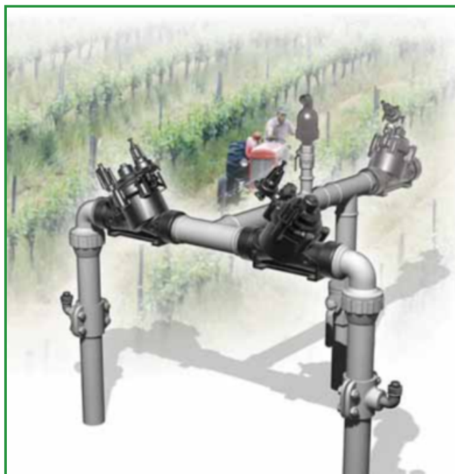
[1] BERMAD Model IR-120-54-b opens upon pressure rise command, and establishes reduced pressure zone protecting laterals and distribution line.
