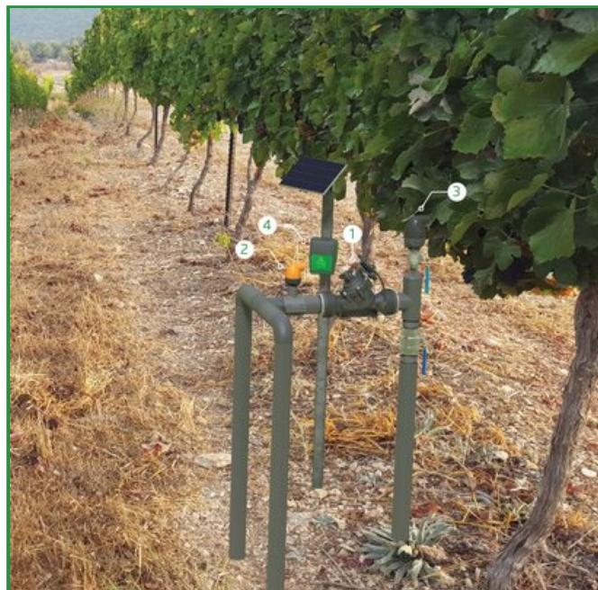
[1] BERMAD Model IR-110-3W-X opens in response to an electric signal.
