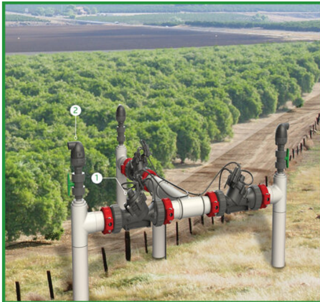
[1] BERMAD Model IR-105-54-3W-X opens upon pressure rise command.
