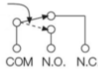
Typical waterflow alarm (increasing system pressure)
