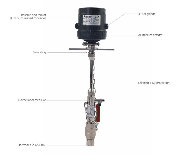
—The electromagnetic insertion flowmeterdesigned for the toughest applications —
