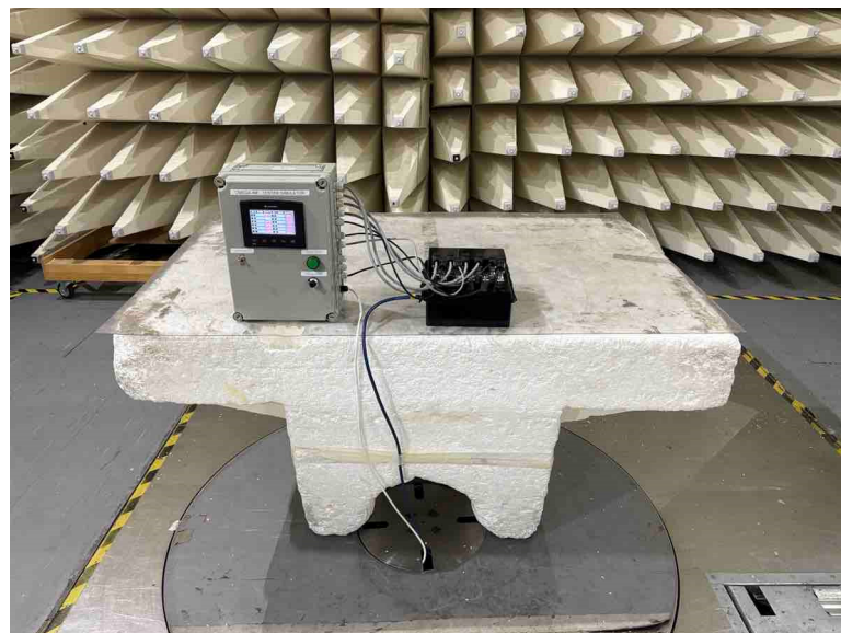
Photograph 7.1.2 Setup for radiated emission measurements, EUT cabling
