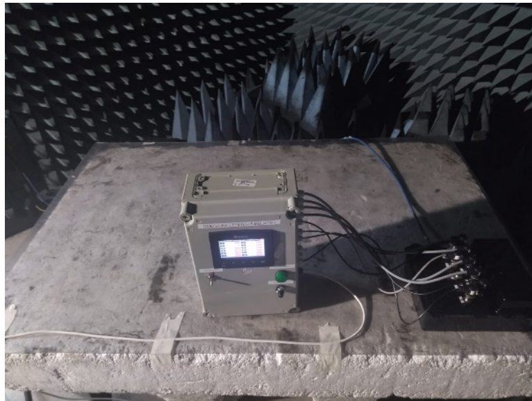
Photograph 8.2.2 Setup for radiated immunity to RF electromagnetic field test, EUT cabling
