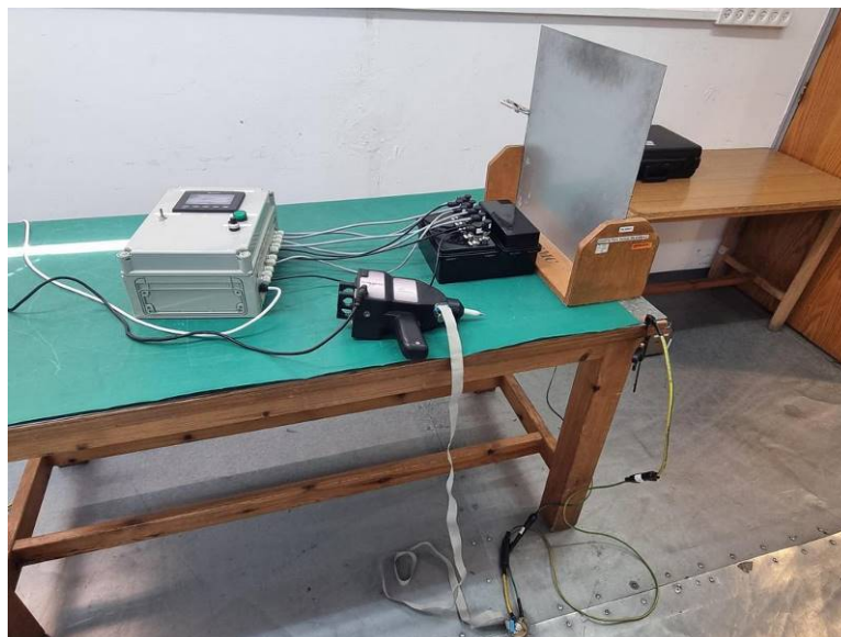
Photograph 8.1.1 Setup for immunity to ESD, general view
