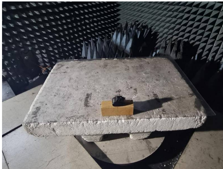
Photograph 8.2.2 Setup for radiated immunity to RF electromagnetic field test, EUT view
