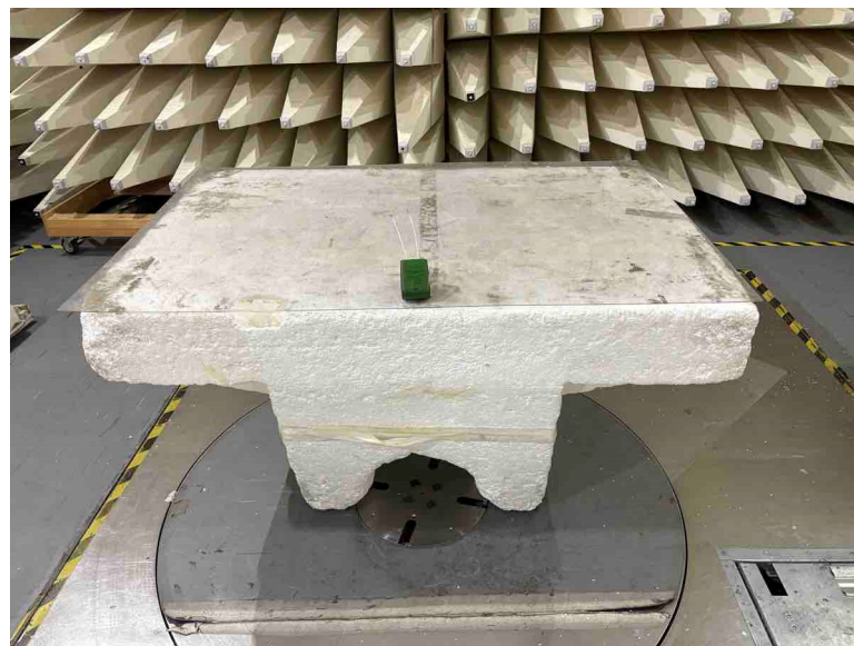
Photograph 7.1.2 Setup for radiated emission measurements, EUT view
