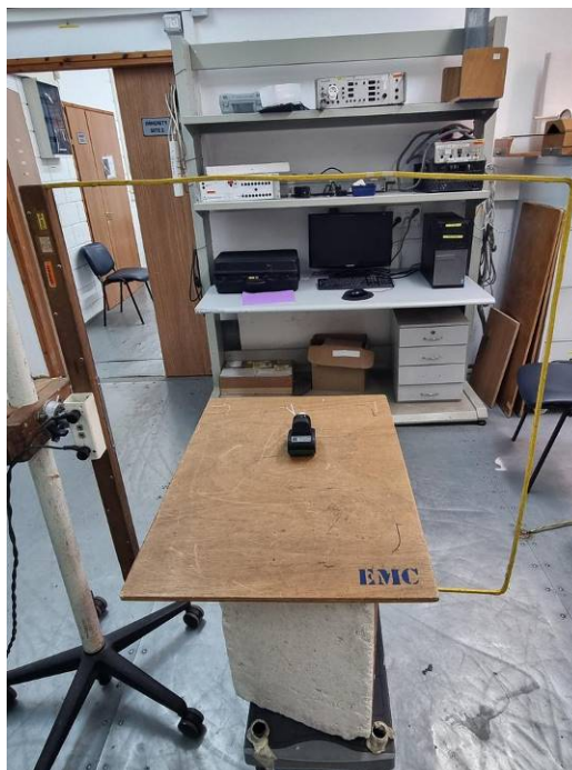
Photograph 8.3.1 Setup for immunity to power frequency magnetic field
