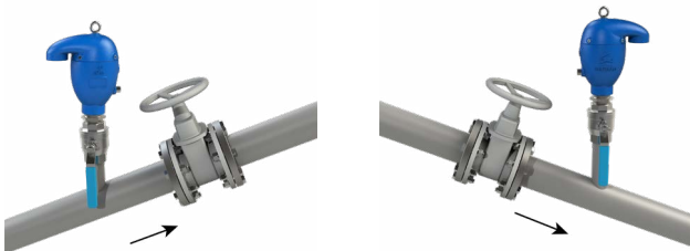
Picture 5.10 – Isolation valve in up / down slope lines
