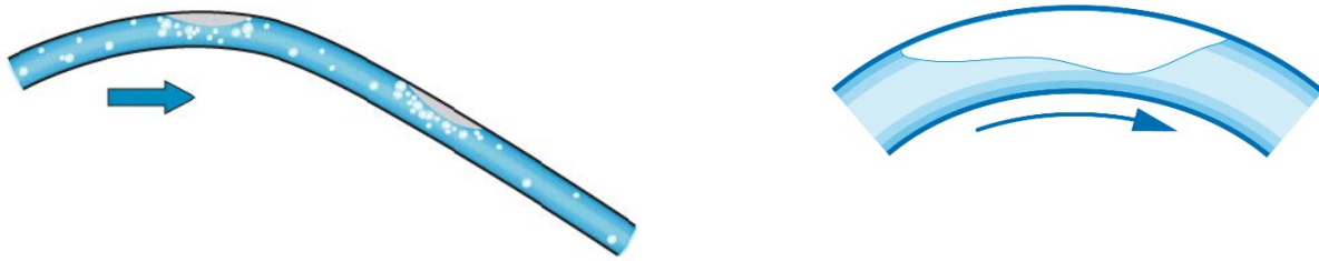
Picture 1.3 - Air bubbles create entrapped air pockets
