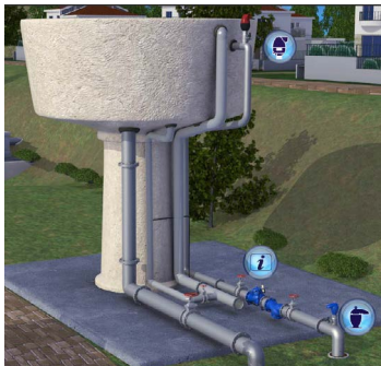
Picture 4.5 - Elevated reservoir
