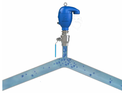
Picture 2.2 - Releasing entrapped air pockets
