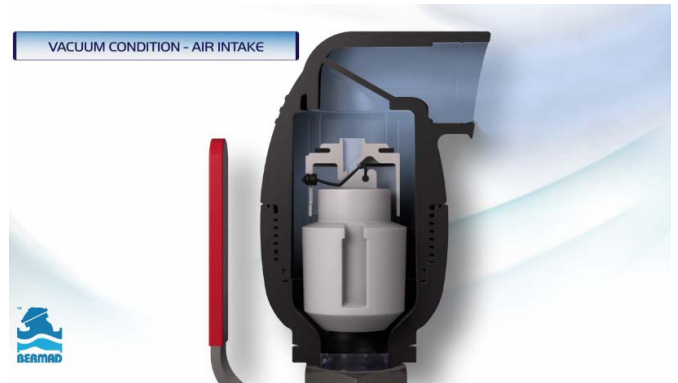
Picture 3.4 C30, Air intake during vacuum conditions
