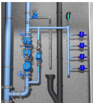
Picture 4.7 - On floor pressure reducing system
