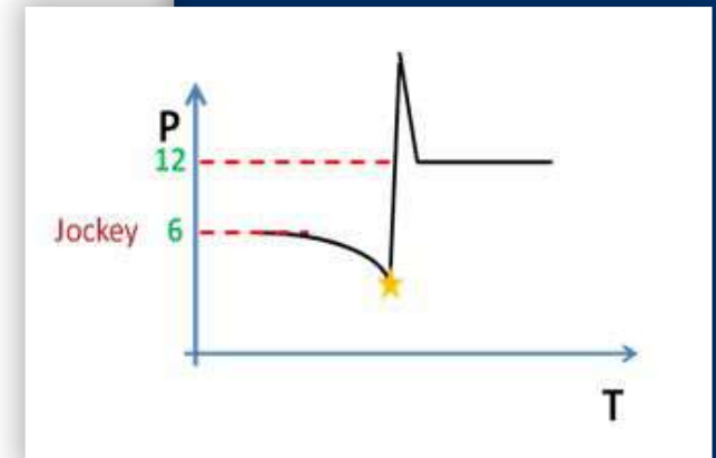
Fig. 4 - Lower jockey pressure setting
