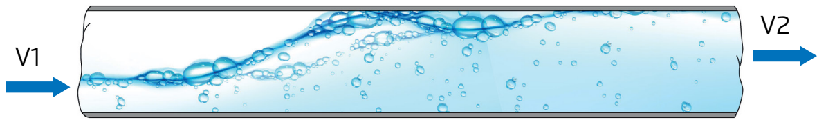
Fig. 31 Air pockets inside the pipe
