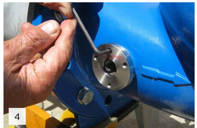
Fasten the fixing screw using 4mm Allen key to prevent the disk from twisting
