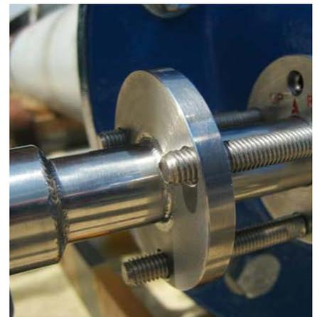
Carefully insert the sensor into the disk, make sure not to damage the O-ring
