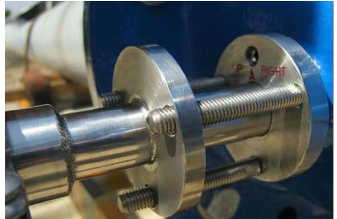
Use the table below to select the correct three 'Short' or 'Long' stud bolt according to the valve DN size. Use the supplied 6mm wrench to screw-in the painted green side of the stud bolt till the stud bolts are locked against their thread end
