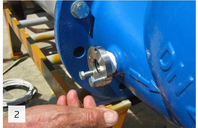
Screw the sealing disk into the 1" BSPT port; use two regular screws to lock the disk temporarily in the up-right position as indicated on the disk. Tighten the disk gently
