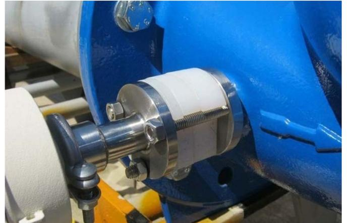
Tighten the nuts but make sure not to apply excessive torque, it may damage the plastic spacer
