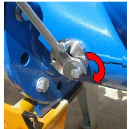
**Important:** do not tie the sealing disk till the very end of its tread; only position it in the up-right position
